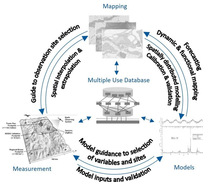
**Figure 4.** Integrative loop of measuring, modeling, mapping, and data mining as an integrated and evolutionary approach to address the complexity and dynamics of environmental systems across scales (modified 3M approach from Lin (2010)).
