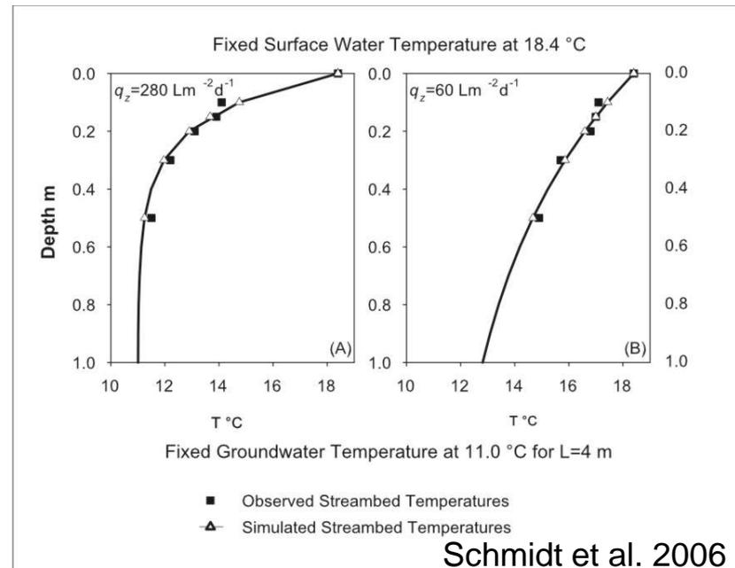
Example temperature profiles with fitted water fluxes
