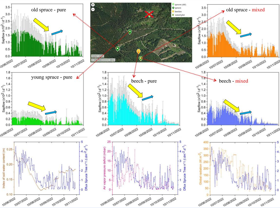
36 trees equipped (pure and mixed plots of spruce & beech trees) – thermal dissipation method [2]
