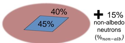
Example of contribution to the count rate of neutrons that originate a) inside the field (45%), b) outside the field (40%), and c) non albedo neutrons (15%)
