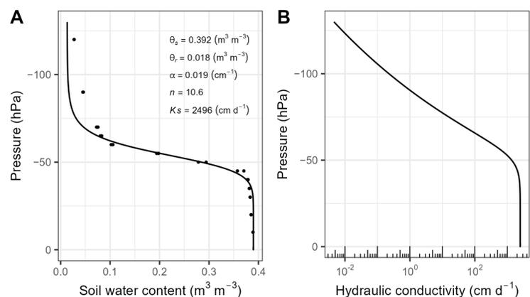
(A) Soil water retention curve and fitting parameters and (B) unsaturated hydraulic conductivity curve of F36 sand estimated with the van Genuchten-Mualem model [4]. For comparability with the sandbox, the data and curves are only shown up to a pressure of 130 hPa.
