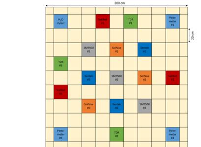
Schematic view of the sensor arrangement in the sandbox.
