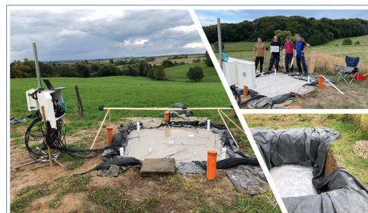
Photos of the sensors and piezometer arrangement in the sandbox experiment
