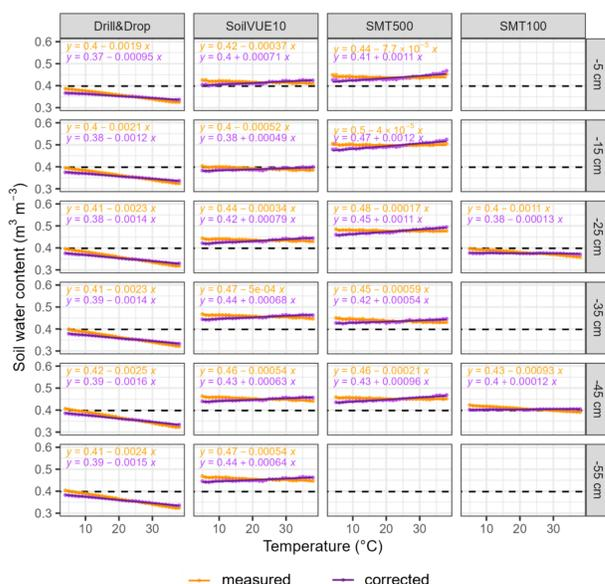
Soil moisture as a function of temperature before and after correction for the temperature effect on the dielectric permittivity of water.
