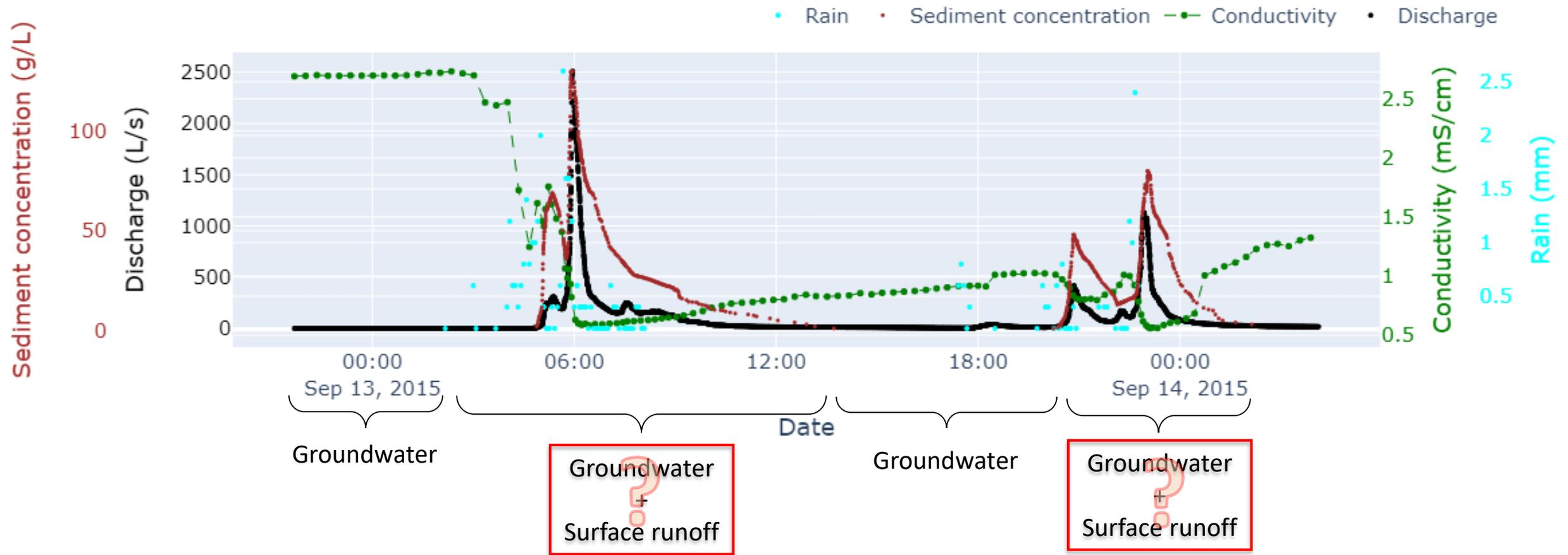
Groundwater more mineralized than surface runoff :  $\chi_G \gg \chi_{SR}$
