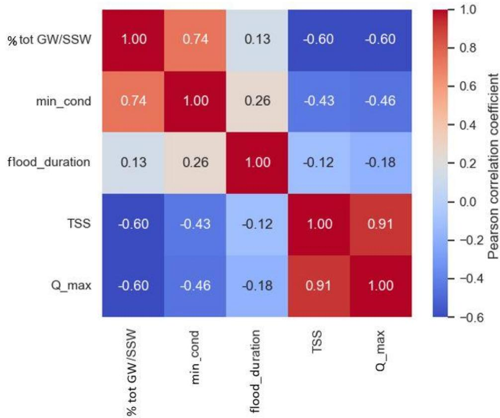
*Pearson correlation coefficients between the flood total groundwater contribution (% tot GW/SSW) and the flood minimum conductivity (min\_cond), duration, total export of sediment (TSS) and maximum discharge ( Q\_max).*
