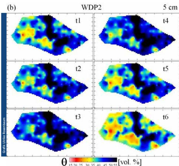
*Spatial distribution of soil moisture within the Wüstabach catchment area at a depth of 5 cm (red: dry; blue: moist). A precipitation event occurred at t1, resulting in significant changes in soil moisture patterns: the pronounced contrast between high soil moisture values along the stream and relatively low values in the slope areas at t1 is reduced during precipitation (until t3). The contrast increases again during the ensuing dry period*
