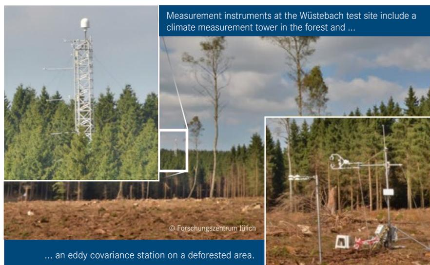
Measurement instruments at the Wüstebach test site include a climate measurement tower in the forest and ...
