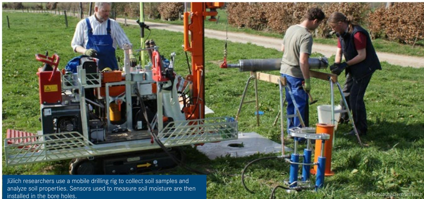
Jülich researchers use a mobile drilling rig to collect soil samples and analyze soil properties. Sensors used to measure soil moisture are then installed in the bore holes.
