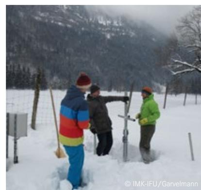
At the Graswang site, installing a SnowFox system to measure cosmic radiation
