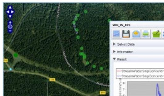
The TERENO Data Discovery Portal displays both the location of the measurement stations (green circles on the map) as well as time series for given parameters.
