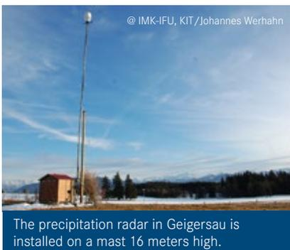
Located on the “Geigersau” farm within TERENO’s Bavarian Alps/pre-Alps observatory, the rainfall radar, operated since 2009 by the Institute of Meteorology and Climate Research (IMK-IFU) at the Karlsruhe Institute of Technology, transmits its data to the TERENO data portal TEODOOR for visualization online. Installed on Mount Kimberg at an elevation of 950 meters, the radar operates on a special short-wave frequency known as X-Band. With 12 scans per minute, the radar can scan precipitation
