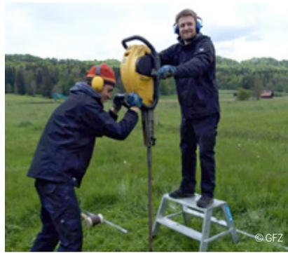
determining a location, for example, we use the signal that enters the sensor directly. But here we use the part of signal that first enters the soil and then the sensor. The signal changes depending on how much water is in the soil, and this allows us to draw inferences about the soil moisture," says Rasche.
