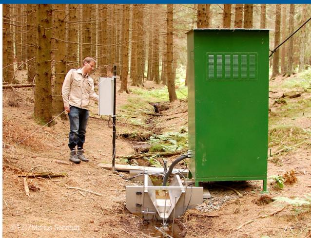
Runoff measurement station at TERENO's Wüstebach site
