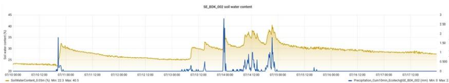
Data from the TERENO site in Selhausen. The blue line shows when and how much rain fell between July 10-17, 2021. The yellow-green line shows how the soil moisture changed as a result of the precipitation during this period.
