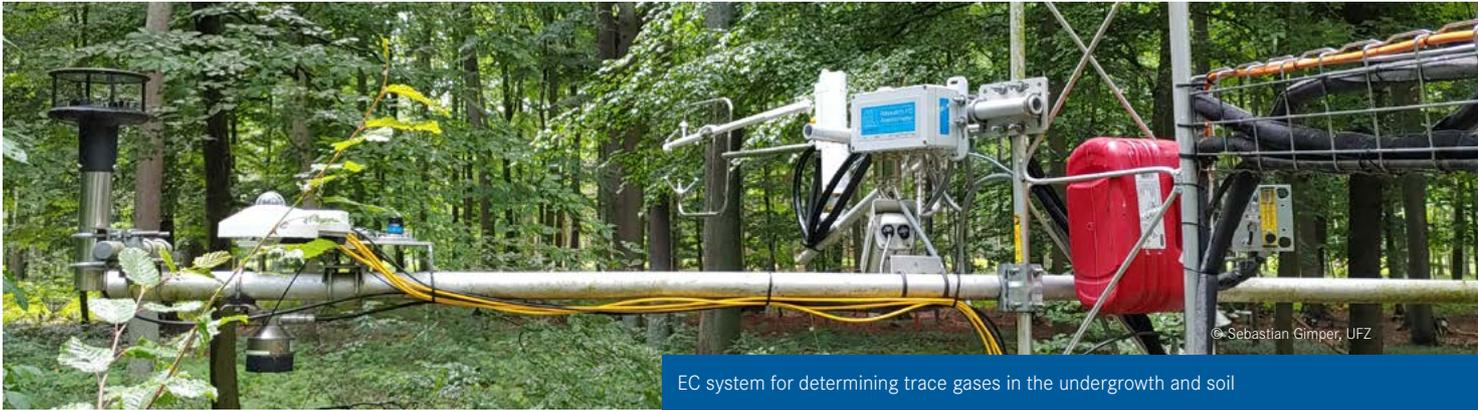
EC system for determining trace gases in the undergrowth and soil
