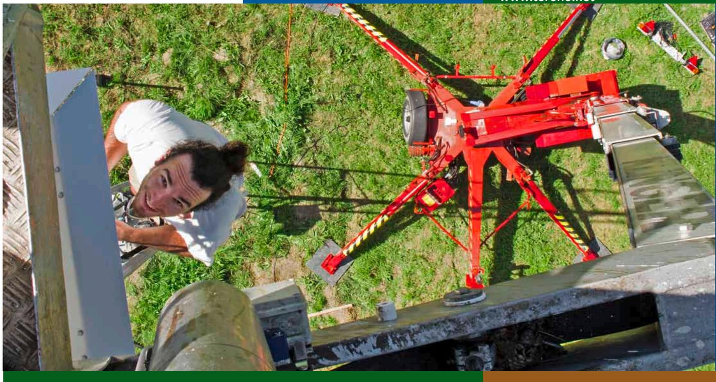
*Aiming high: Christian Chwala from the Karlsruhe Institute of Technology (KIT) installs a self-developed measuring device at the Fendt test site that uses microwave radiation to test new methods for collecting precipitation and humidity data*
