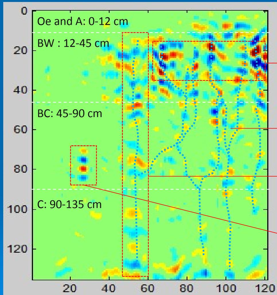
Near-surface lateral macropore flow and vertical finger flow
