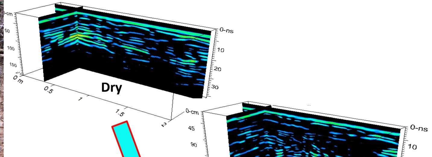
**Time-lapsed GPR in combination with real-time soil water monitoring have revealed flow paths in ... fractured shales and the impacts of soil layering on subsurface lateral flow**
