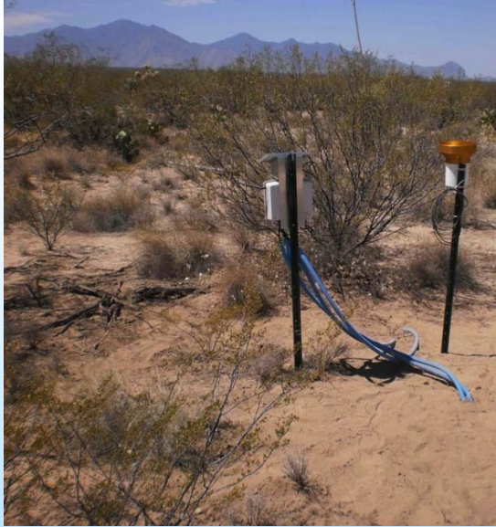
Tipping bucket rain gauge, Santa Rita, Arizona, USA.
