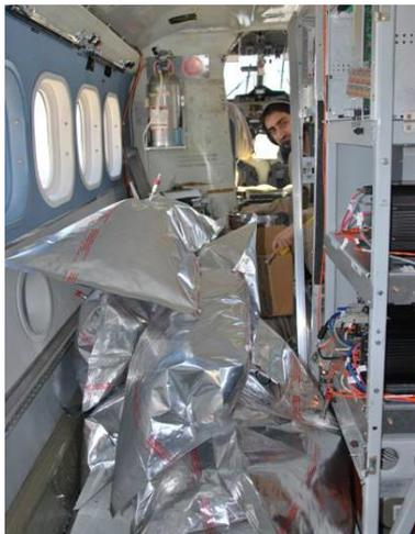
in-flight REA sample collection & post-flight REA sample analysis using Picarro G1301
