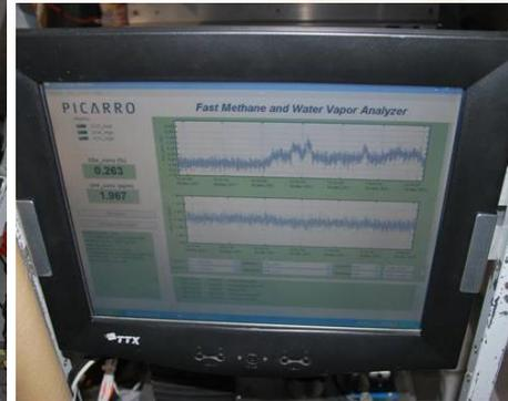
CH<sub>4</sub> Analyzer (G2301) and real-time display
