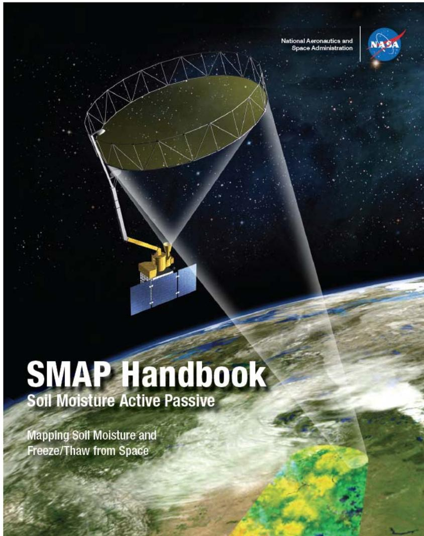
L-band unfocused SAR and radiometer system, offset-fed 6 m light-weight deployable mesh reflector.
